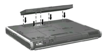
Inserting the battery pack tabs into the battery bay recesses
